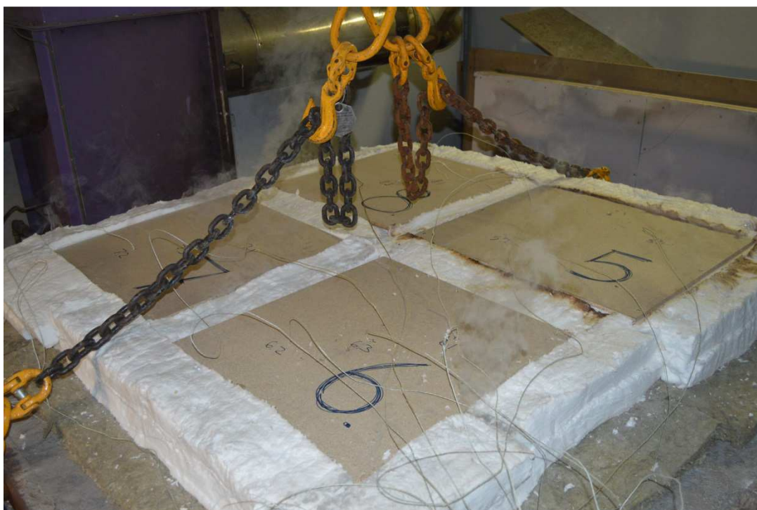
Photo No. 9 Test specimens no 5,6,7 and 8 after 3 minutes of testing
