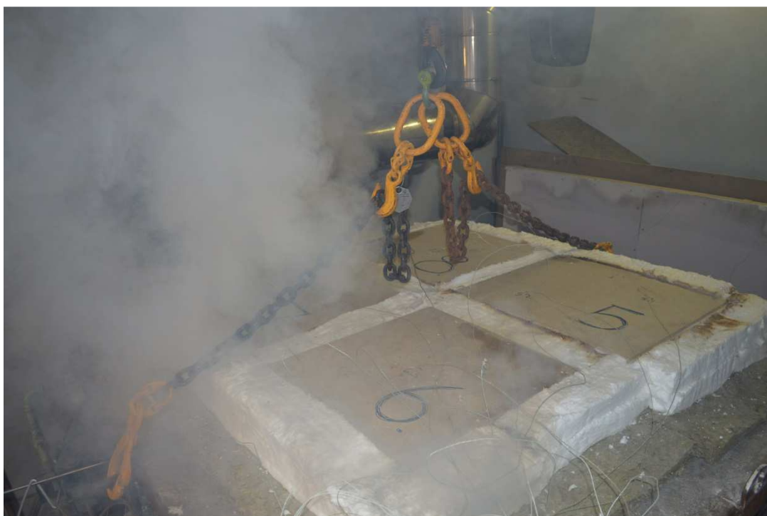
Photo No. 11 Test specimens no 5,6,7 and 8 after 9 minutes of testing
