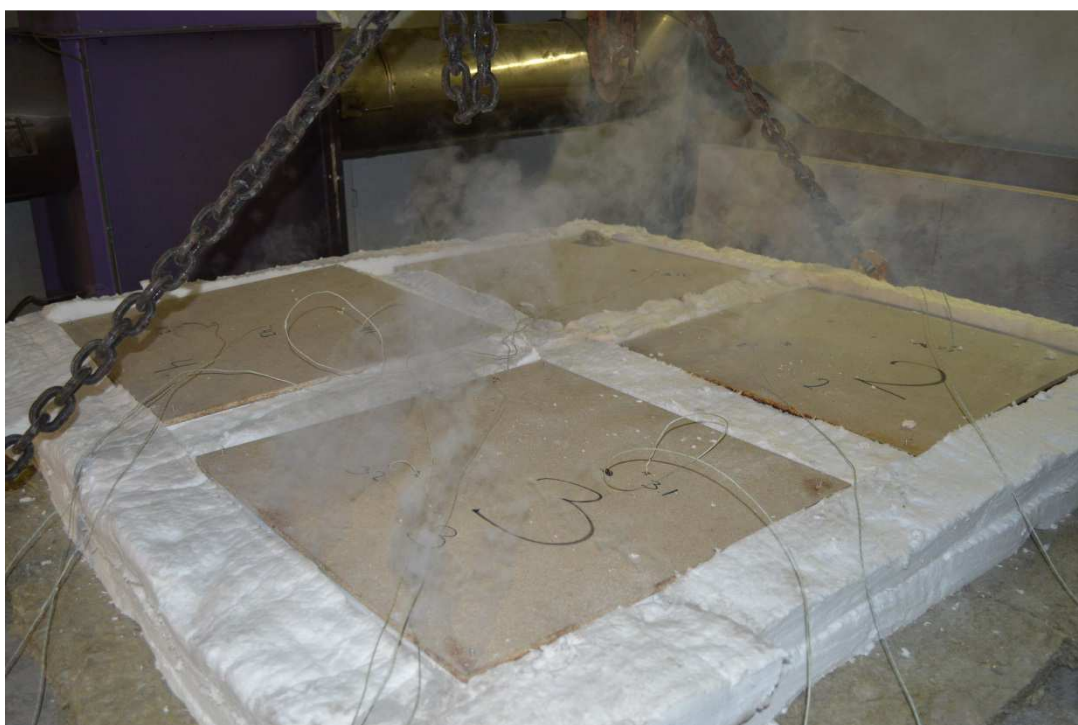
Photo No. 4 Test specimens no 1,2,3 and 4 after 7 minutes of testing
