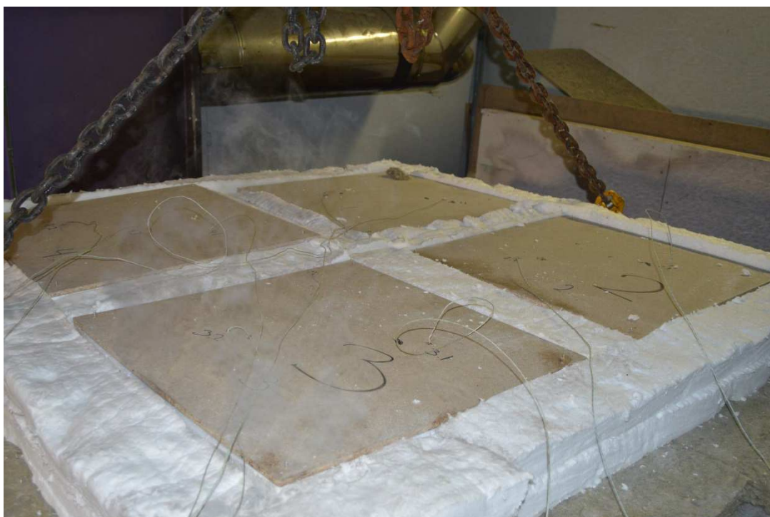
Photo No. 3 Test specimens no 1,2,3 and 4 after 6 minutes of testing
