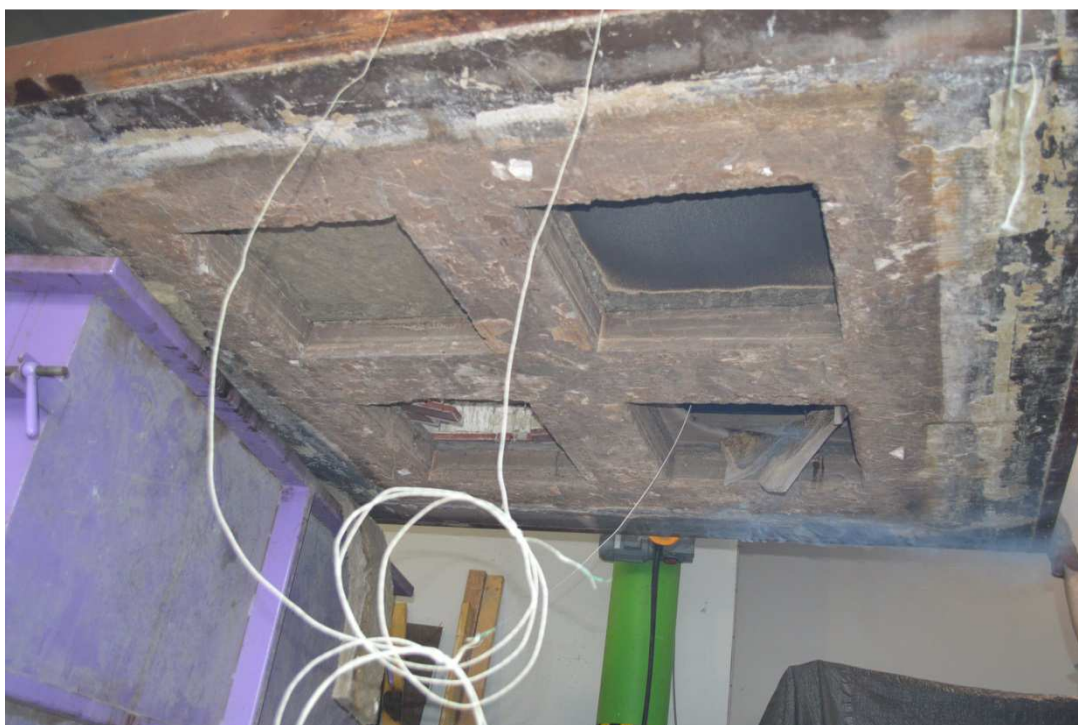
Photo No. 5 Test specimens no 1,2,3 and 4 from exposed side after the test
