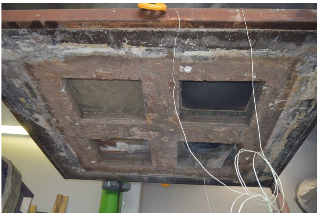
Photo No. 6 Test specimens no 1,2,3 and 4 from exposed side after the test
